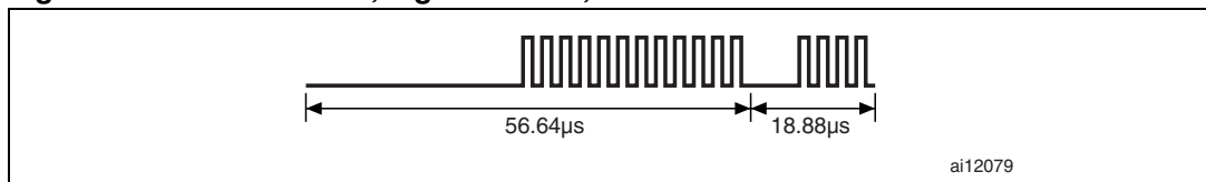
Figure 24. Start of frame, high data rate, one subcarrier x2
